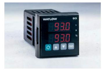
The SERIES 93 is a microprocessor-based controller with single input and dual output. It has a feature set that includes heat/cool auto tune, ramp to set point, versatile alarms and percent power limit. Optional hardware features include red or green displays, universal low and high voltage power supply, CE compliance and a NEMA 4X rating.
