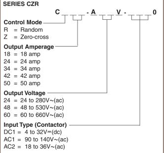
**Note:** Do not use the AC1 and AC2 input type models with temperature control outputs that include an AC snubber filter. This could cause the CZR to stay full on.
